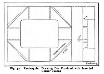
the use of expensive steel, such as high-speed steel, for these corner pieces. This form of die is not recommended for small work. The particular die illustrated was designed for drawing steel parts 6 by 8 inches in size and it has outworn several sets of corner pieces.
